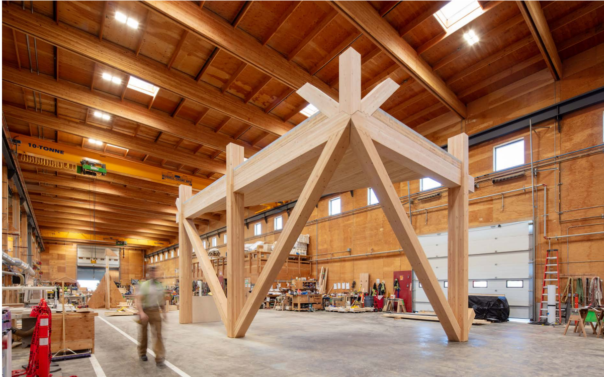
A FULL-SCALE MOCK-UP OF THE ALL-WOOD DIAGRID WAS BUILT
