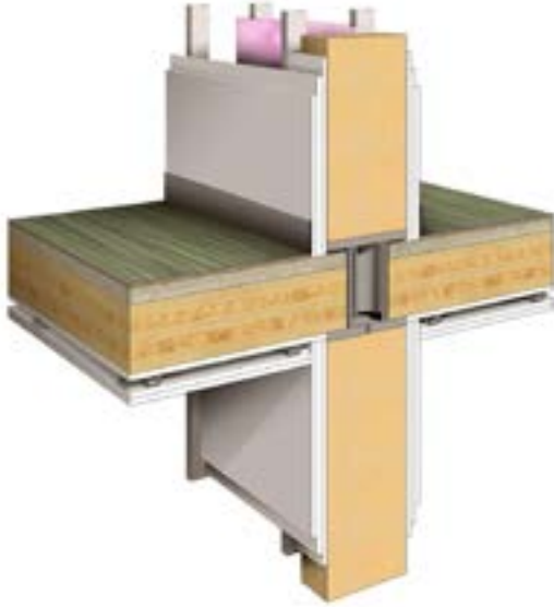
FIGURE 5.28: END-GRAIN TO END-GRAIN COLUMN CONNECTIONS MINIMIZE SHRINKAGE
