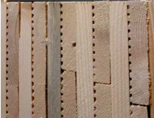
FIGURE 4: A SECTION OF MHM SHOWING LONGITUDINAL GROOVES IN LAMINATIONS INTENDED TO ENHANCE THE THERMAL-INSULATION PROPERTIES OF THE PANELS [19] (A) AND A DOWEL LAMINATED PANEL SHOWING THE 60-DEGREE LAYER
