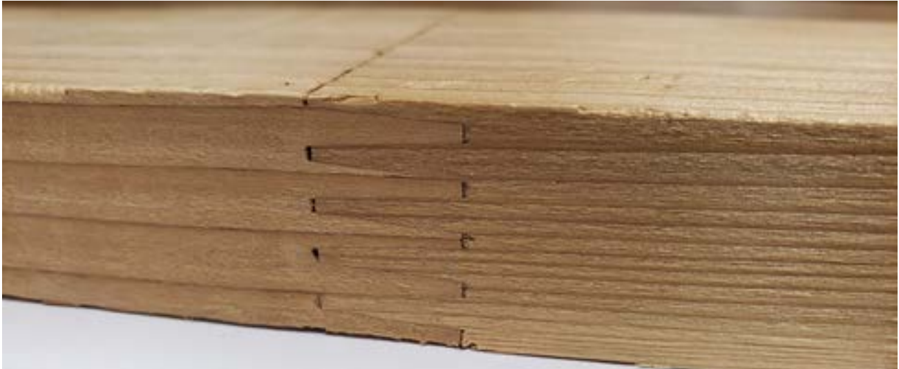
FIGURE 4.1: ILLUSTRATION OF FINGER-JOINTED LUMBER
