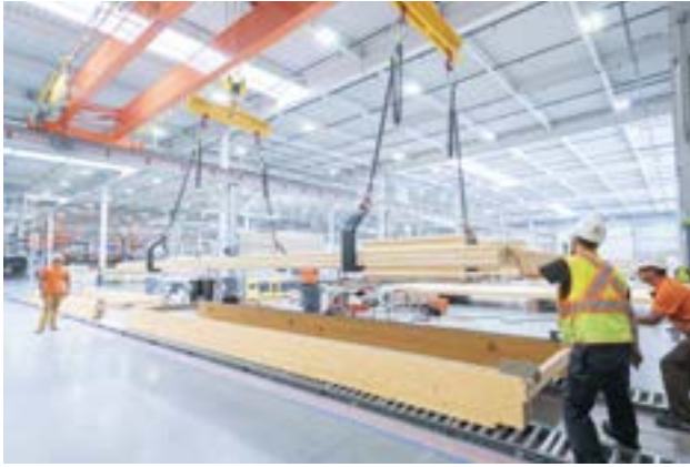
FIGURE 6.6: ASSEMBLING PREFABRICATED COMPONENTS IN A FACTORY SETTING
