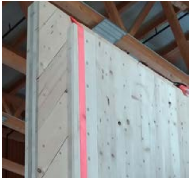
FIGURE 4: A SECTION OF MHM SHOWING LONGITUDINAL GROOVES IN LAMINATIONS INTENDED TO ENHANCE THE THERMAL-INSULATION PROPERTIES OF THE PANELS [19] (A) AND A DOWEL LAMINATED PANEL SHOWING THE 60-DEGREE LAYER
