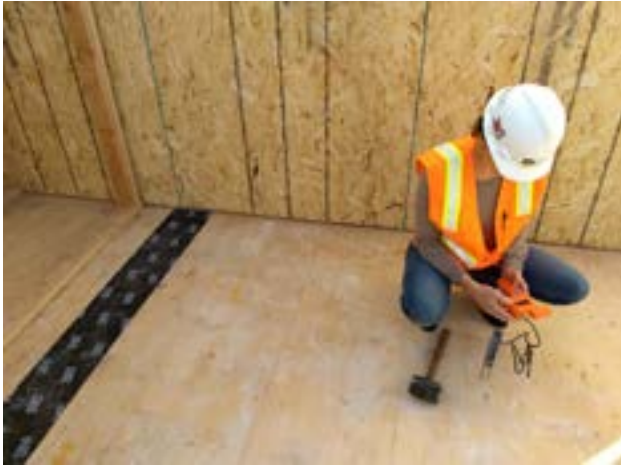
FIGURE 5.27: MOISTURE MONITORING CLT FLOORS WITH A HAMMER-IN PROBE
