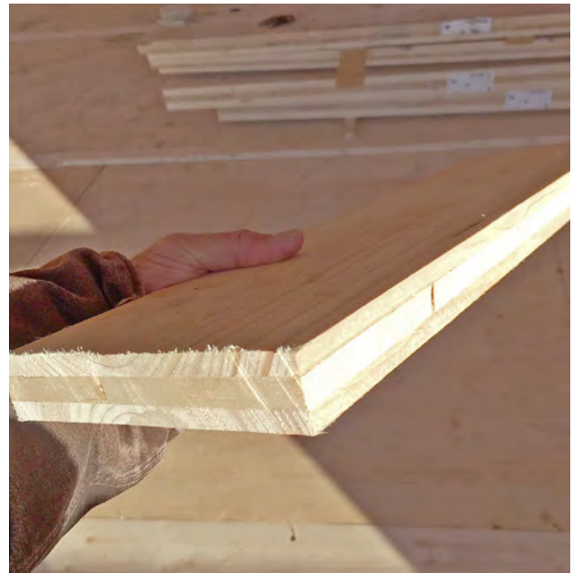
FIGURE 5.11: SPLINE CONNECTION MATERIAL EXAMPLES: PLYWOOD AND JOINERY BOARD
