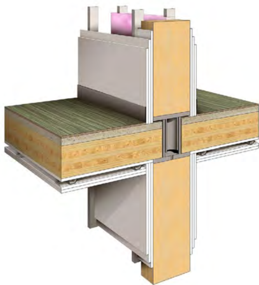
FIGURE 5.29: END-GRAIN TO END-GRAIN COLUMN CONNECTIONS MINIMIZE SHRINKAGE
