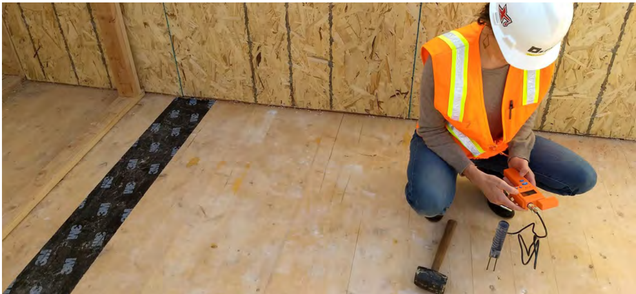
FIGURE 5.28: MOISTURE MONITORING CLT FLOORS WITH A HAMMER-IN PROBE
