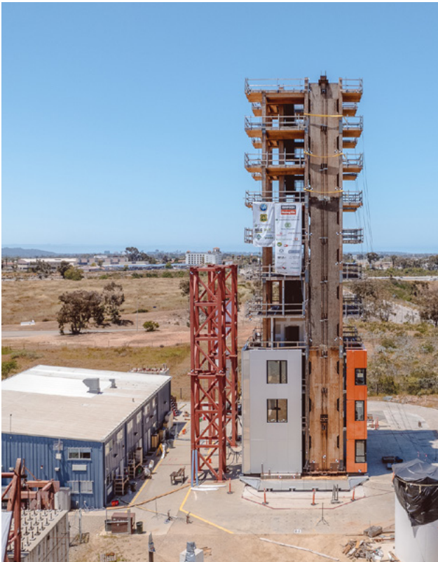
FIGURE 5.42: 10-STORY TIMBER TOWER EARTHQUAKE TEST NHERI Shake Table, 2023 Source: Timberlab/FLOR
