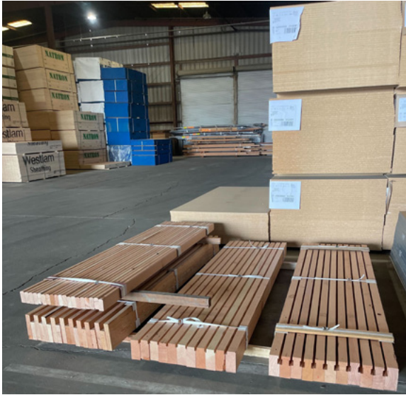
DLT MADE WITH RECLAIMED WOOD, READY FOR ASSEMBLY
