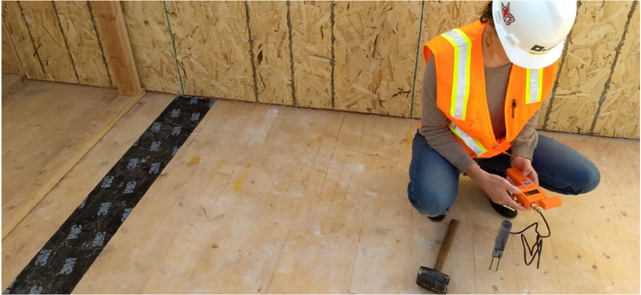
FIGURE 5.29: MOISTURE MONITORING CLT FLOORS WITH A HAMMER-IN PROBE
