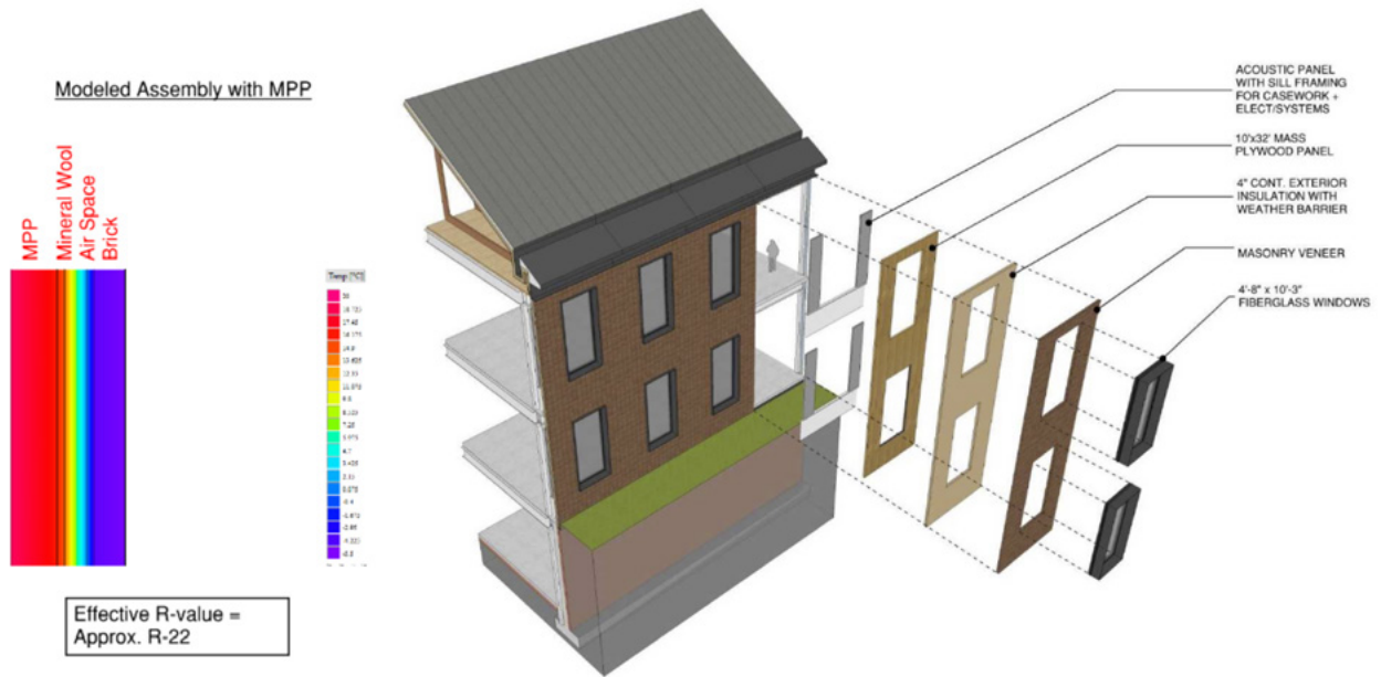
FIGURE 5.28: MPP WALL ASSEMBLY FOR IMPROVED THERMAL RESISTANCE
