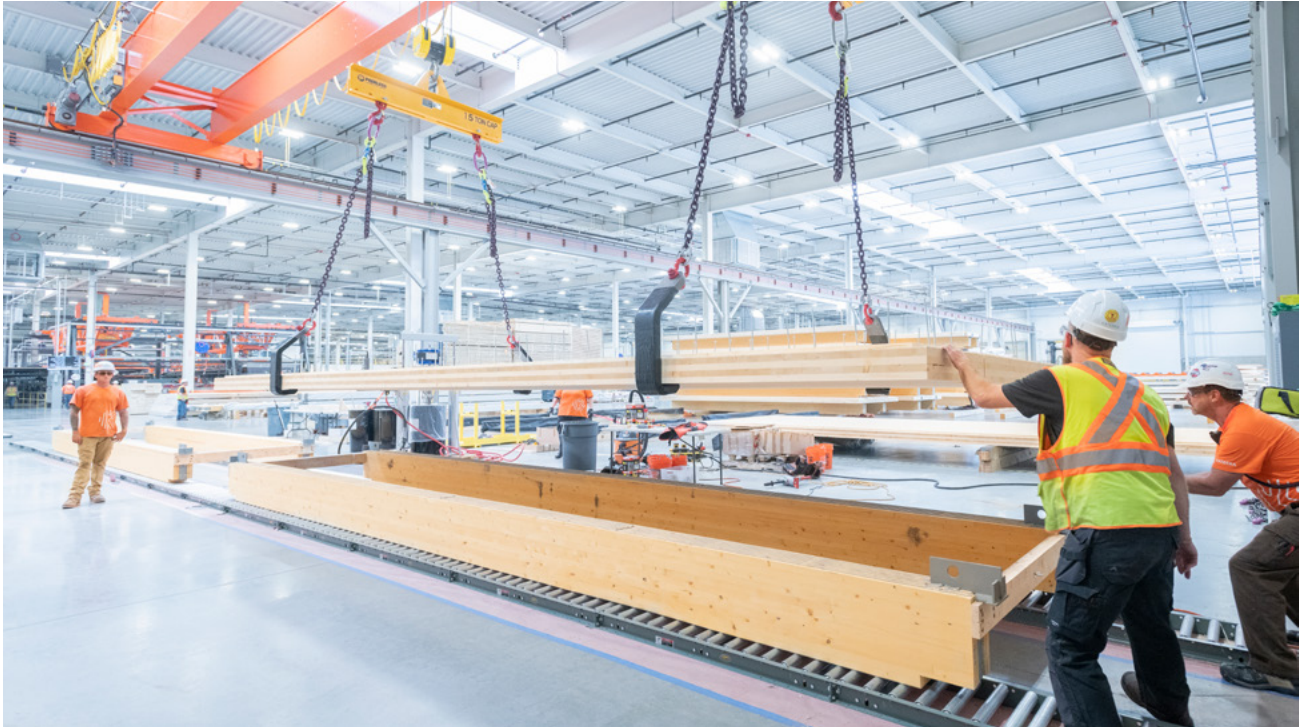
FIGURE 6.9: ASSEMBLING PREFABRICATED COMPONENTS IN A FACTORY SETTING
