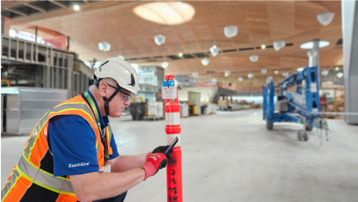
A POLYGON EMPLOYEE CHECKS REAL-TIME T/RH LEVELS, USING THE EXACTAIRE REMOTE MONITORING MOBILE APP
