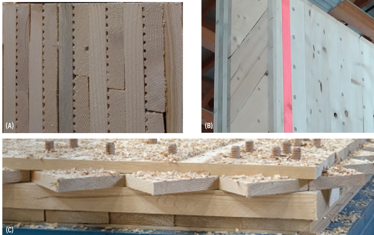
FIGURE 10.3: THREE EXAMPLES OF CROSS-LAMINATED PANELS BONDED WITH NAILS AND DOWELS: (A) A SECTION OF SOLID WOOD WALL SHOWING LONGITUDINAL GROOVES IN LAMINATIONS INTENDED TO ENHANCE THE THERMAL-INSULATION PROPERTIES OF THE PANELS [17], (B) A DOWEL-LAMINATED WOOD100 PANEL SHOWING THE 60-DEGREE LAYER (SOURCE: L. MUSZYNSKI), AND (C) CONSTRUCTION OF ROMBACH NUR-HOLZ PRODUCT WITH THREADED HARDWOOD DOWELS AND A 45-DEGREE LAYER (SECOND FROM THE TOP) [24].
