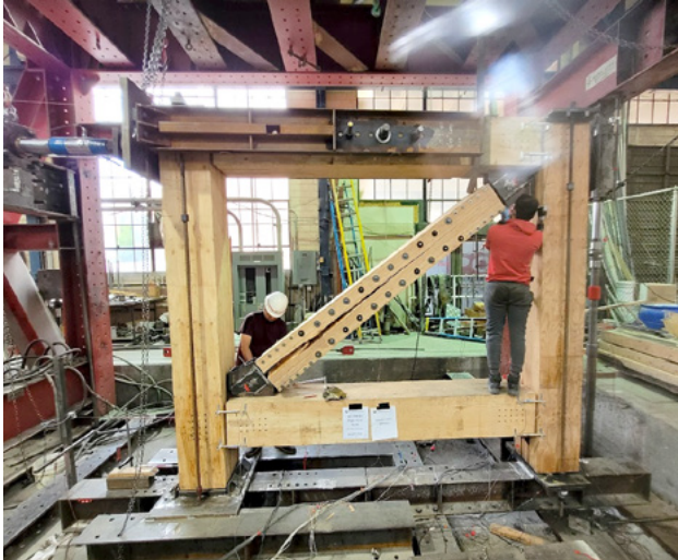
TOP — FIGURE 5.23: CLT AND GLULAM STRUCTURE WITH BRB FRAME CORE AND MPP STAIR
