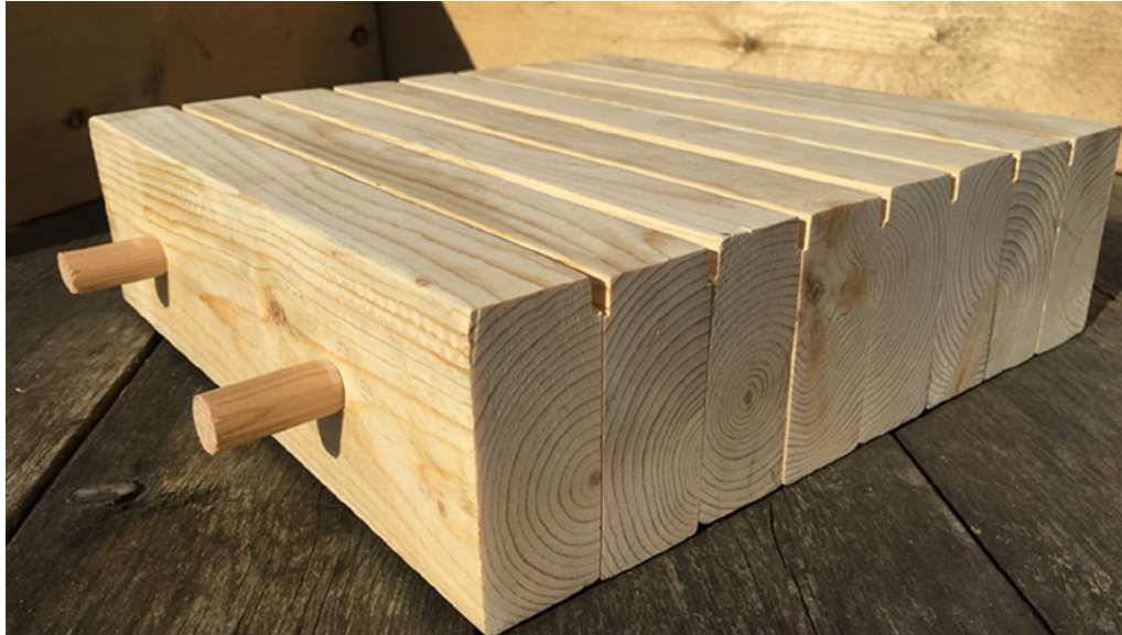
FIGURE 1.4 DOWEL-LAMINATED TIMBER (DLT) PANEL
