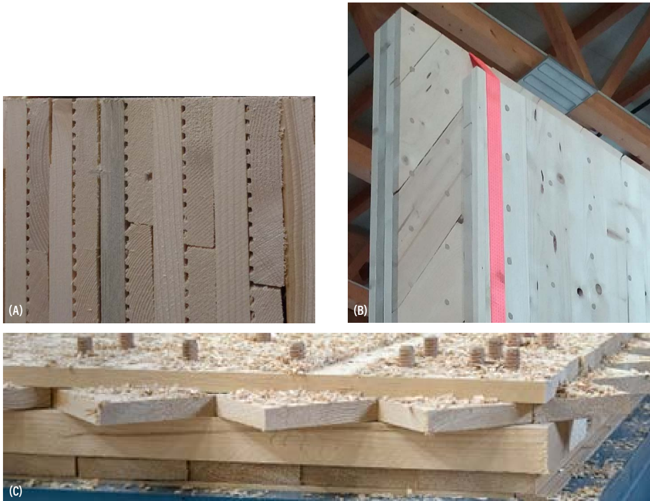
FIGURE 10.3: THREE EXAMPLES OF CROSS-LAMINATED PANELS BONDED WITH NAILS AND DOWELS: (A) A SECTION OF SOLID WOOD WALL SHOWING LONGITUDINAL GROOVES IN LAMINATIONS INTENDED TO ENHANCE THE THERMAL-INSULATION PROPERTIES OF THE PANELS*, (B) A DOWEL-LAMINATED WOOD100 PANEL SHOWING THE 60-DEGREE LAYER (SOURCE: L. MUSZYŃSKI), AND (C) CONSTRUCTION OF ROMBACH NUR-HOLZ PRODUCT WITH THREADED HARDWOOD DOWELS AND A 45-DEGREE LAYER (SECOND FROM THE TOP) **
