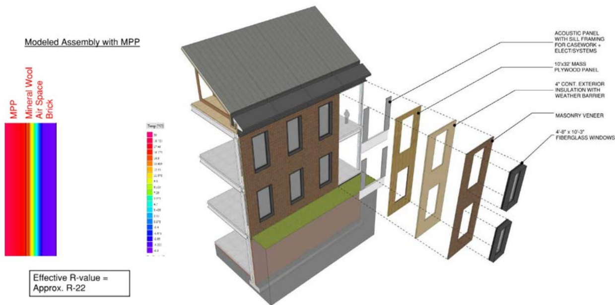
FIGURE 5.28: MPP WALL ASSEMBLY FOR IMPROVED THERMAL RESISTANCE
