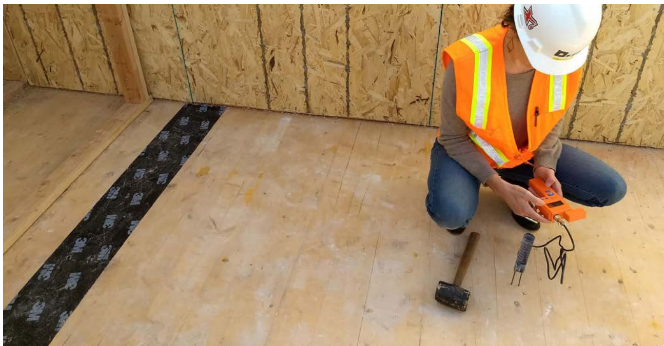
FIGURE 5.29: MOISTURE MONITORING IN CLT FLOORS WITH A HAMMER-IN PROBE
