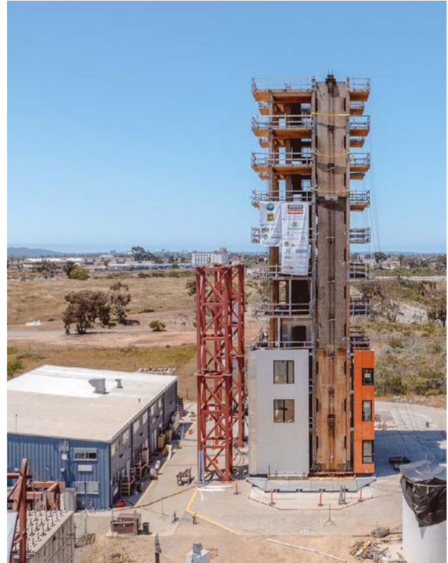
FIGURE 5.42: 10-STORY TIMBER TOWER EARTHQUAKE TEST
